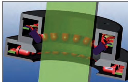
Customer-specific light in sectional view
