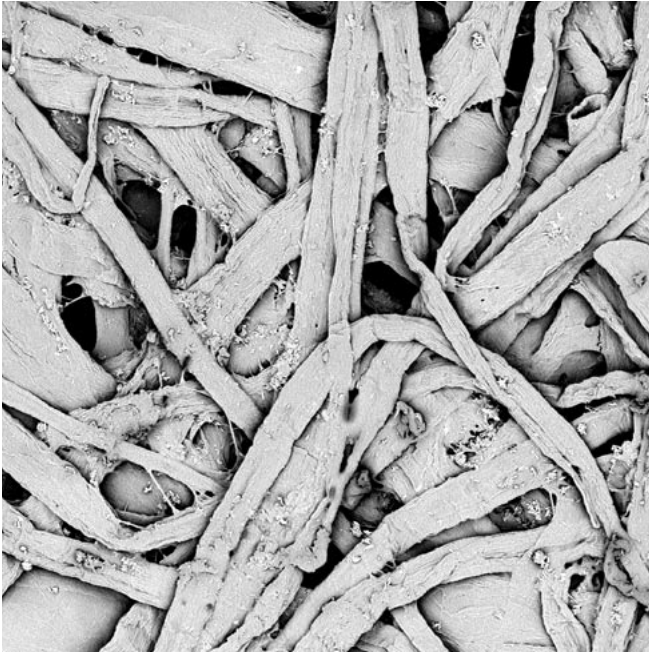
Image of regular printer paper showing individual fibers. Magnification 830x, field of view 240 \mu\text{m} .
