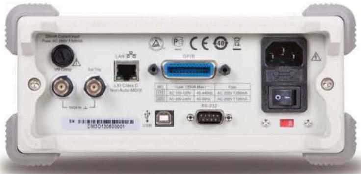
Standard interfaces: USB Host, USB Device, RS-232, GPIB, LAN (LXI-C)
