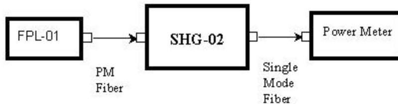
SHG-02 Power Conversion Measurement Setup
