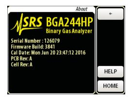
After about 15 seconds the Gas Purity Analyzer Home page will appear. Assuming the unit has come from the factory and the gas port caps haven't been removed, it should display <0.1% deviation reading for Argon.
