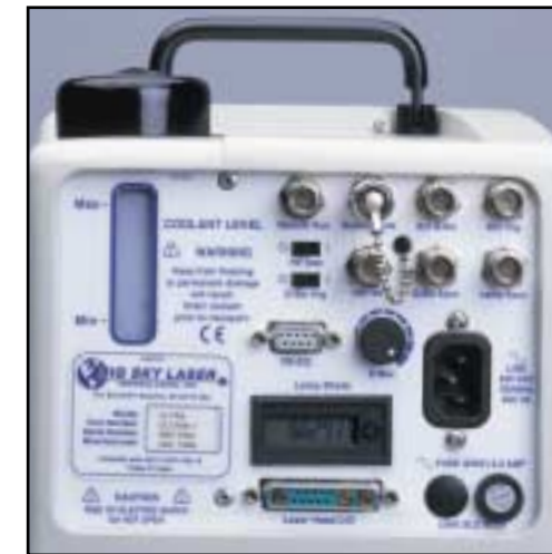
Easy access to synchronization I/O, RS232 interface, shots counter, water level...
