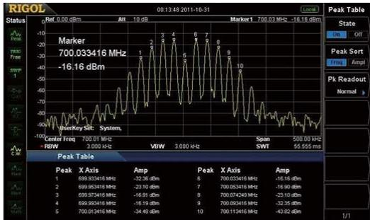
Measure lower level signal with the preamplifier turn on
