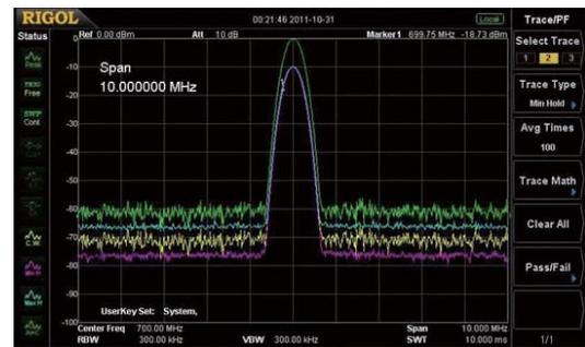
Readout the spectrum peak values with the peak table function
