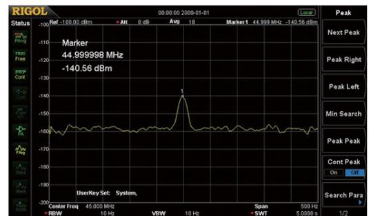
Phase noise < -80 dBc/Hz @10 kHz offset
