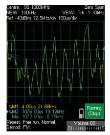
In addition to audio demodulation of AM or FM signals, the modulating waveform can be displayed against a timebase settable between 5us/div and 20ms/div.
