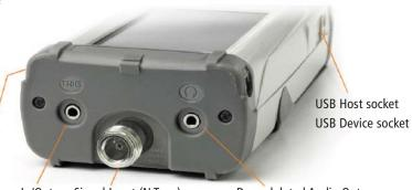
Trigger In/Out Signal Input (N Type)
