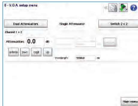
Single attenuator mode: - 60 dB total attenuation - Shutter function
