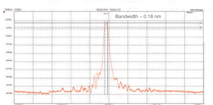
Optical transmission spectrum of AP3380A C-band Tunable filter
