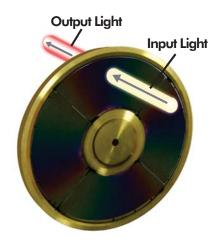
CI Systems' Circular Variable Filters (CVF's) are interference narrow-pass filters of advanced design which are deposited on circular substrates, called segments. Film thickness, and therefore the wavelength of peak transmittance varies linearly and continuously with angular position on the segment.
