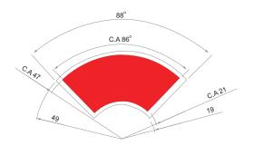
The red area indicates the active filter area or Clear Aperture (C.A). The linear radii dimensions are in millimeters.
