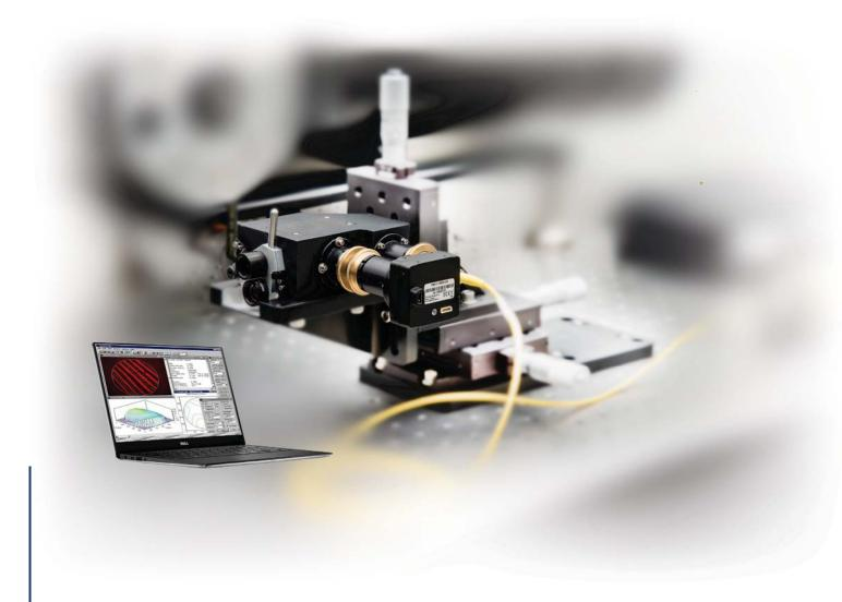
The Laser Unequal Pathlength Interferometer (LUPI) is an ultra compact Twyman-Green interferometer designed for alignment and measurement of reflective or refractive optical systems.
