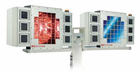
The IRTS-II is a medium to long-range electro-optical missile threat simulator for testing missile approach warning systems and training crew in the operation of these systems. It simulates the IR radiation profile of an approaching missile, based on input parameters such as: missile signature, atmospheric conditions, missile speed, missile range and more.
