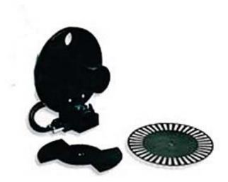
A variable frequency radiation modulator, the SR-600 is a high performance chopper for many applications, including IR jammer simulation and low-level radiation detection. Designed to be robust and flexible, the SR-600 uses interchangeable blades for various chopping frequency ranges. You can operate the SR-600 as a stand-alone unit or mount it to other CI products, such as the SR-200 cavity blackbodies or the ILET90 collimator.
