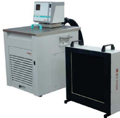
Figure 4: Blackbody head and refrigerator SR-800N-12A-LT
