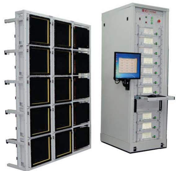
Figure 10: "NUC Tower" System with 15 controlled temperature blackbodies
