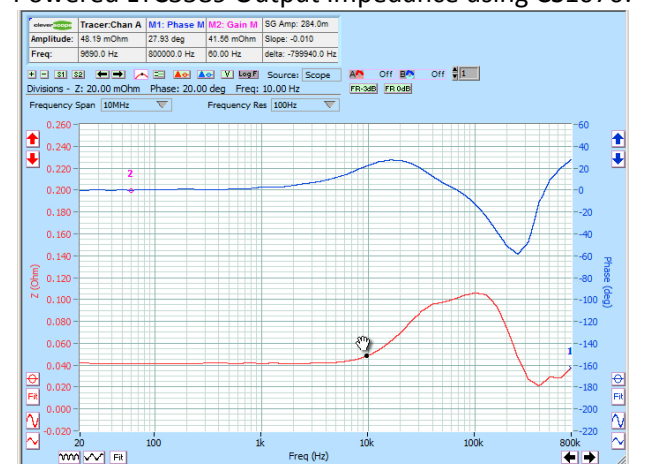
Powered LTC3589 Output Impedance using CS1070:
