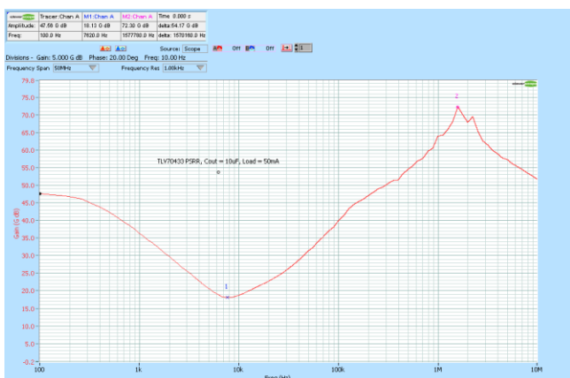
TLV70433 PSRR using CS1070 (1A 50 MHz op-amp):
