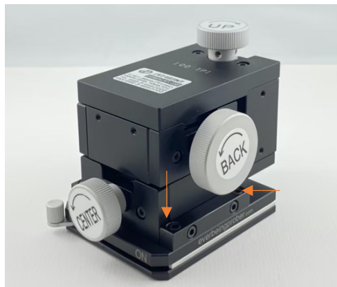
Figure 3. Base screw positions for EB-005(same on opposite side)
