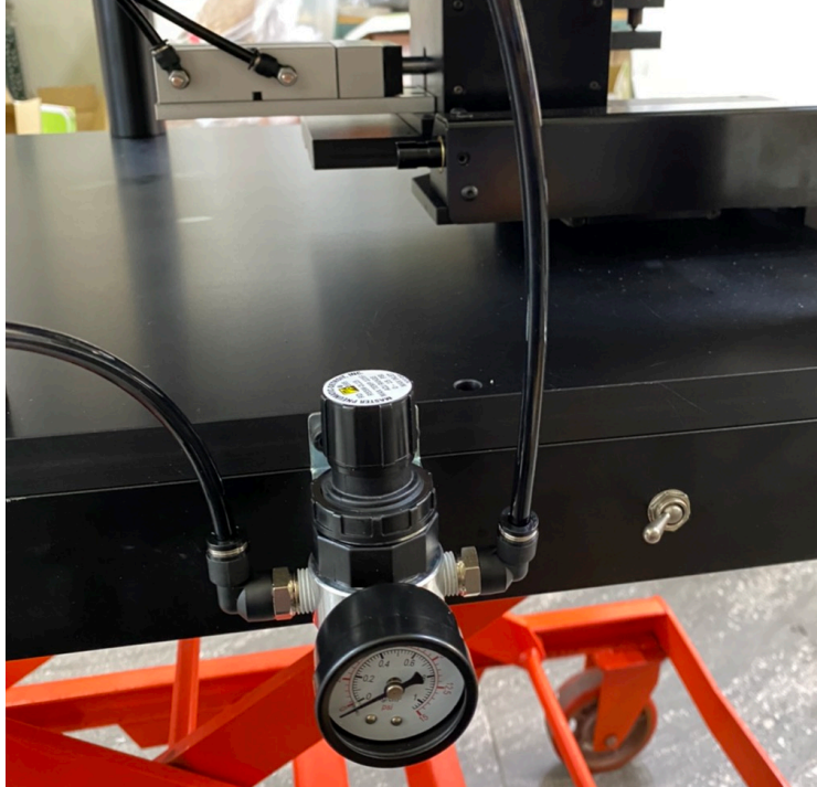
Figure 2. Image of the air regulator for pneumatic chuck lift
