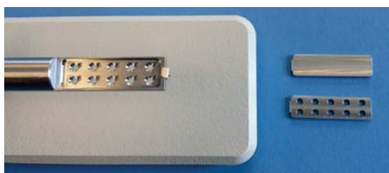
Figure 3. Grid Specimen Holder tip (left) with retaining clip options; single-side exposure (top right) and double-side exposure (bottom right).
