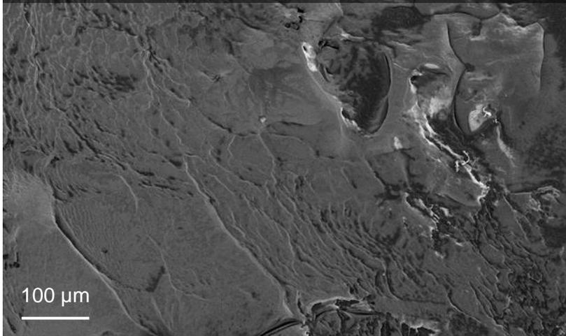
Thermal damage is observed
