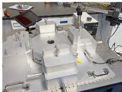
■ Custom Externally Adjustable Probe Station, 50mm × 50mm Sample Stage, for Wafer Electrode Testing
