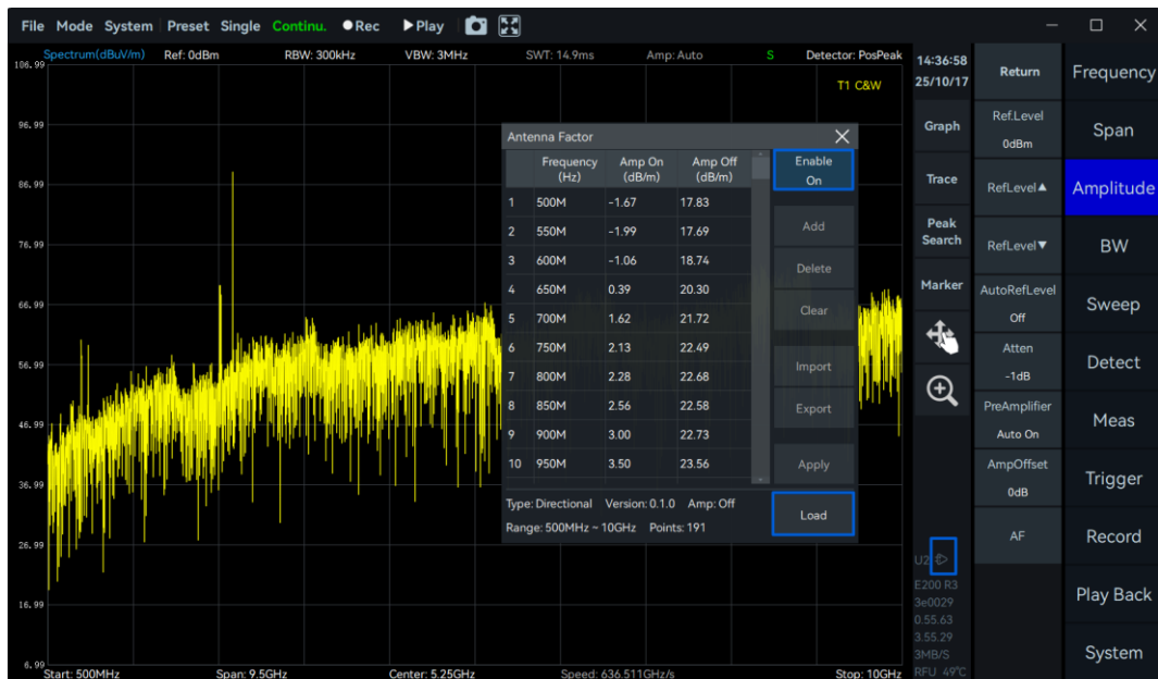
Figure 25 With HDA-100: automatic loading of antenna factors
