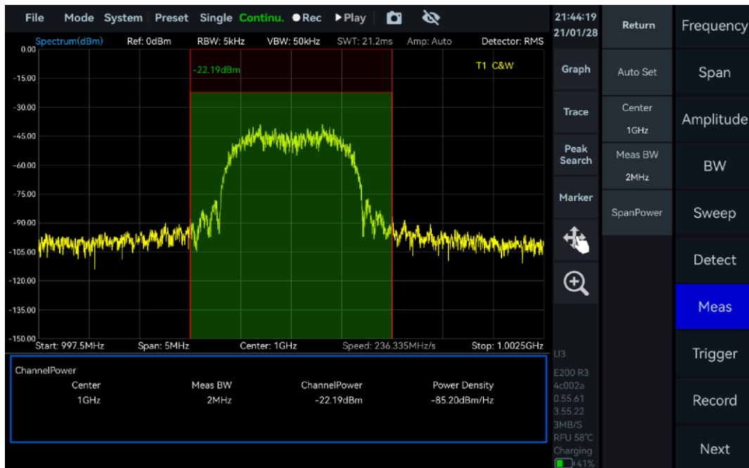
Figure 18 Measurement of ChannelPower
