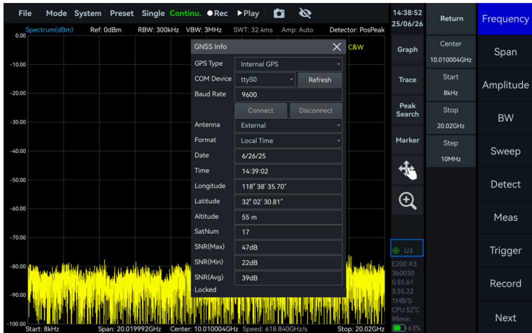
Figure 5 Locked GNSS external antenna
