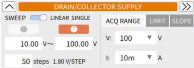
Figure 3.14: DRAIN / COLLECTOR SUPPLY Screen
