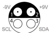
Probe's power supply pin assignment “cable view”
