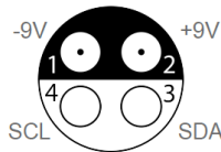
Probe’s power supply pin assignment “cable view”
