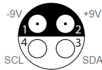
Probe's power supply pin assignment "cable view"
