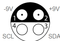
Probe's power supply pin assignment "cable view"
