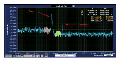
Use convenient cursor tools to measure and examine scatter level and reflection events to measure RL and IL for closely spaced events.
