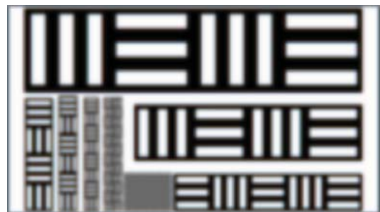
Resolv4K Zoom @ 4.5X High Mag 8.9MP Sensor – 0.76\mu\text{m} / pixel 3.56mm FOV – 5.20\text{mm}^2 Area (3.25X more)
