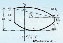
Geometric Parameters: Vertex-to-Vertex Offset (V<sub>1</sub>-V<sub>2</sub>) Wedge Angle (θ<sub>w</sub>) Center Thickness (CT) Edge Thickness Variation (ET<sub>1</sub>-ET<sub>2</sub>) Radius of Curvature (R<sub>1</sub> & R<sub>2</sub>) Sag (Sag<sub>1</sub> & Sag<sub>2</sub>)
