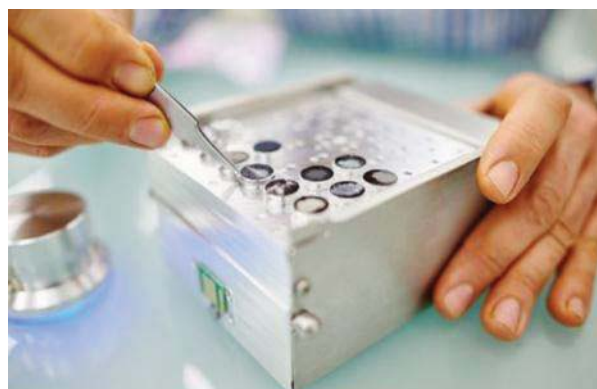
Fig. 20 Sample holder of Phenom XL with pin stubs being loaded
