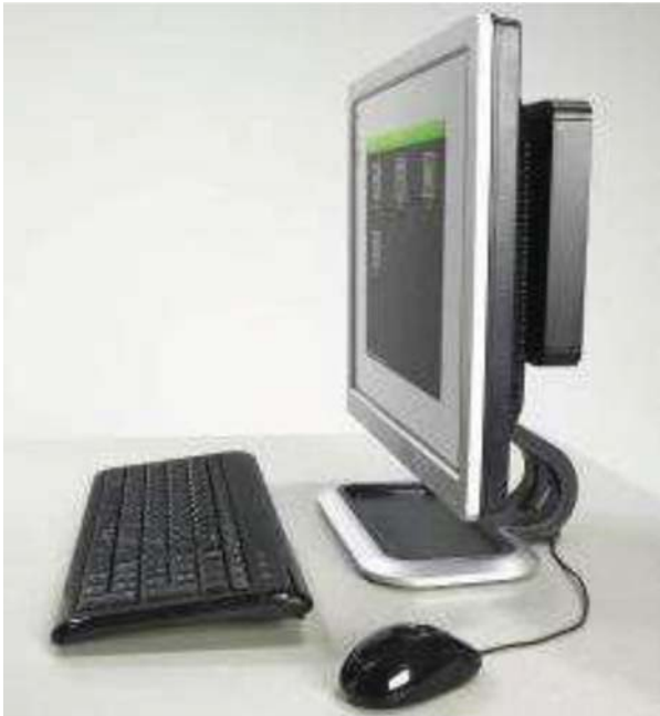
Fig. 35 Side profile of Phenom ProSuite: PC and router are mounted on the back of the monitor
