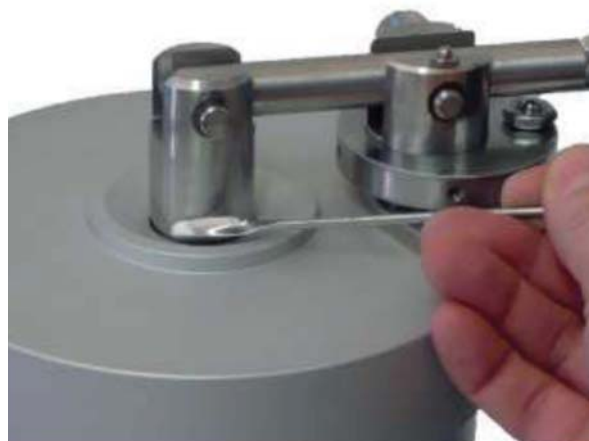
Fig. 44 The powder is unloaded for the inlet valve
