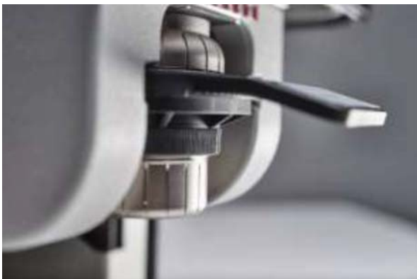
Fig. 23 The sample holder is loaded into the Phenom SEM either Phenom Pure, Pro, and Pro X
