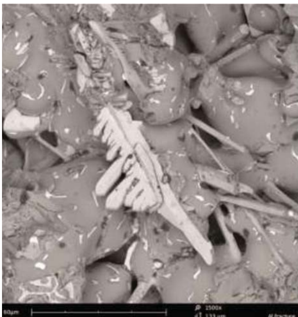
Fig.34 Left: Fracture surface of aluminium at 1500x magnification Right: Butterfly wings at 75,000 magnification
