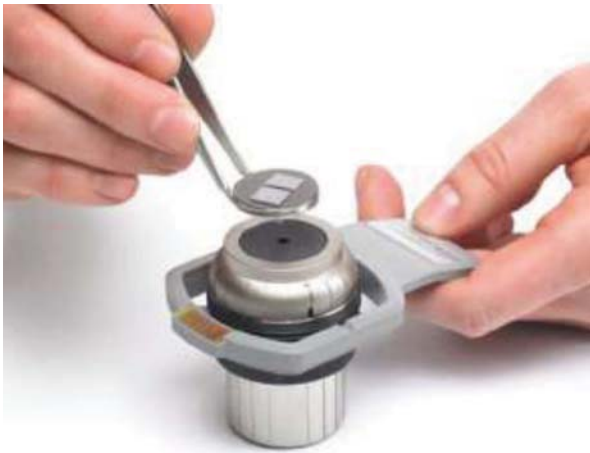
Fig. 22 25mm pin stub with two samples is mounted onto the Phenom sample holder
