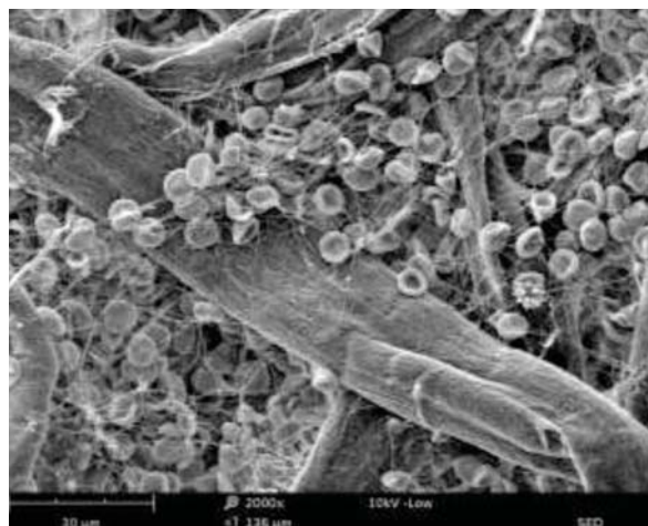
Fig. 12 Topography contrast (SE) platelets with fibrin thread
