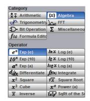
The PicoScope 9400 Series scopes support up to four simultaneous mathematical combinations or functional transformations of acquired waveforms.
