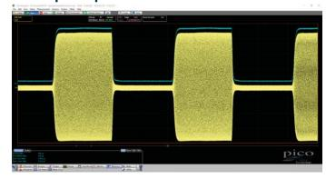
Pulsed RF carriers lie at the heart of our modern communications infrastructures, yet the shape, aberrations and timings of the final carrier pulse (at an antenna, for example) can be challenging to measure. If we choose demodulation, we are subject to the limitations of the demodulator; its bandwidth and distortions.
