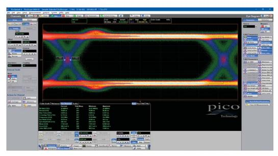
Eye-diagram analysis can be made even more powerful with the addition of mask testing, as described below.
