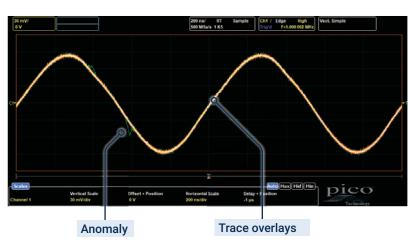
Having captured an anomalous event you can scroll through, or close gates around, an ever smaller block of overlaid traces, until the anomalous trace or traces are found. There is also a segment finder which uses a binary search method to address larger numbers of trace segments:
