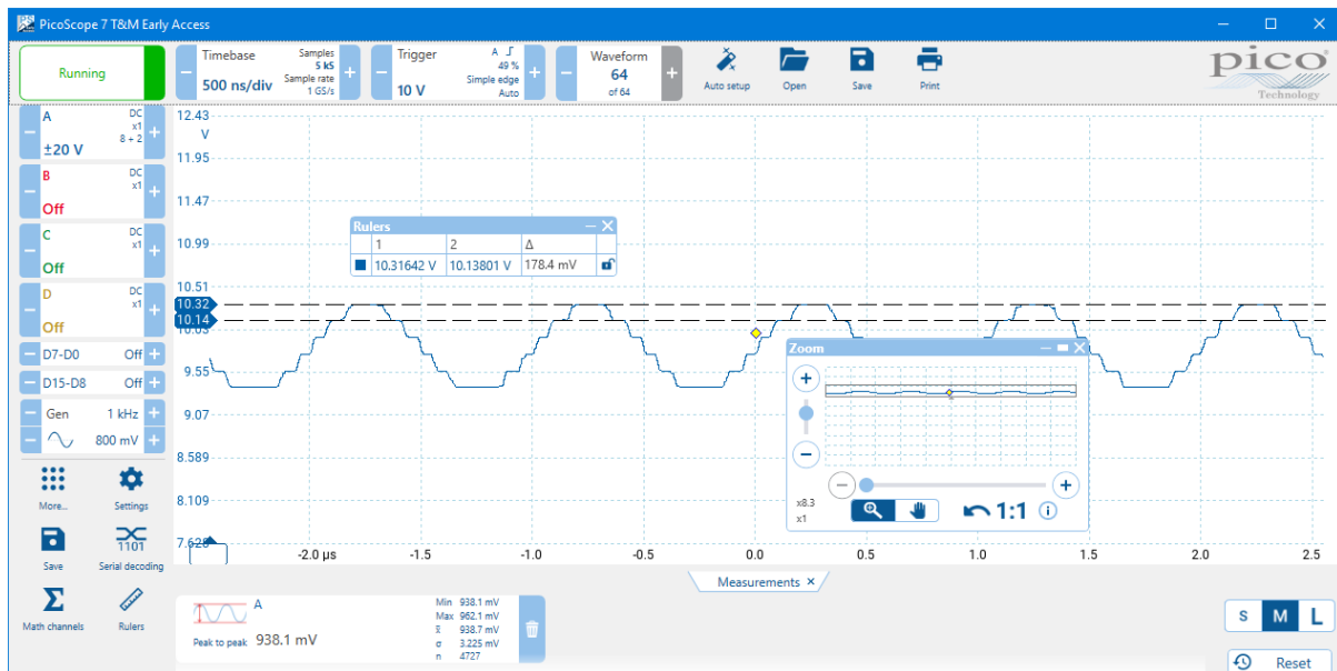
Figure 12 - 1 V p-p sine wave with +10 V offset captured on \pm 20 V range, zoomed in.
