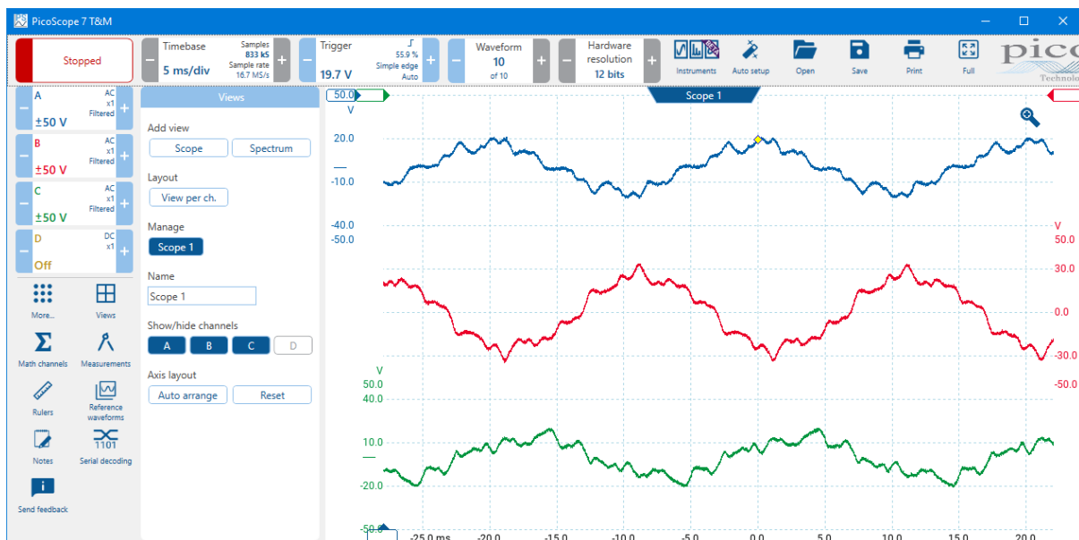
Figure 11 - Three channels with auto-arrange. Note that the input ranges haven't changed and so accuracy and resolution are unaffected.
