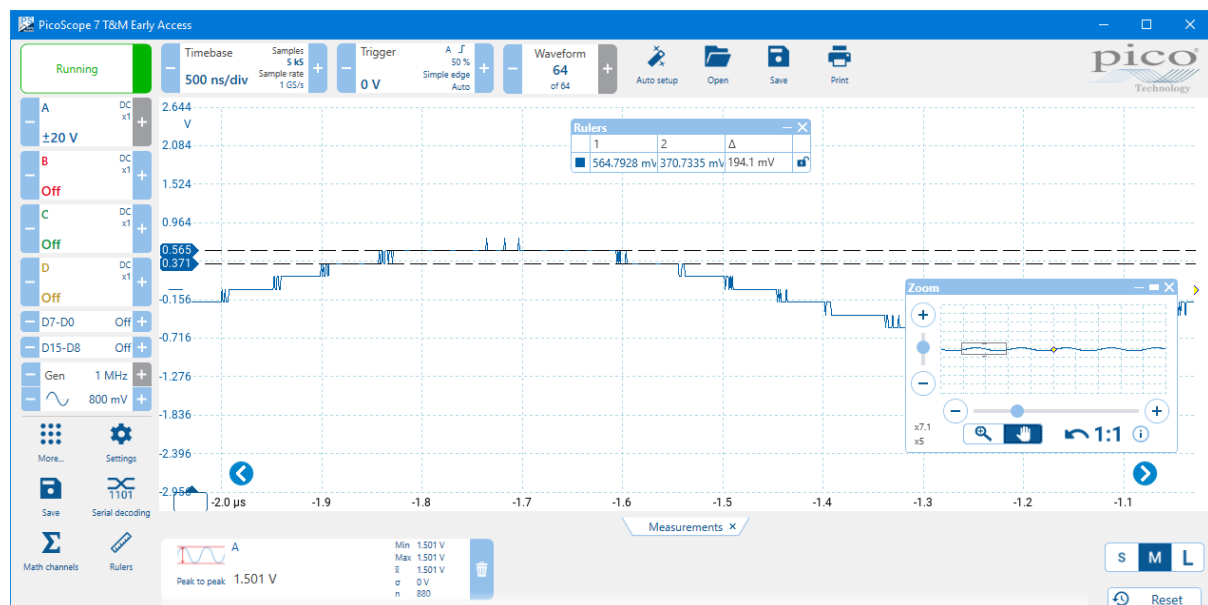
Figure 8 – Sub-1-volt signal on \pm 20 V range. Voltage steps are about 190 mV.
