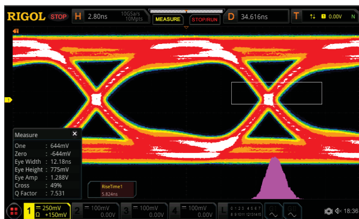
Figure 12: Eye Diagram with improved timing
