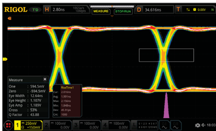
Figure 14: Eye Diagram after debugging and improvements
