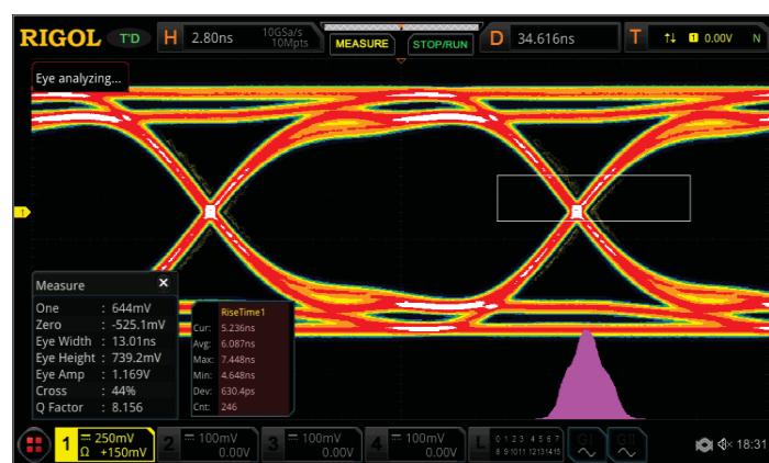
Figure 13: Eye Diagram with improved noise
