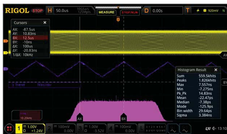
Figure 4: TIE trend and TIE Histogram
