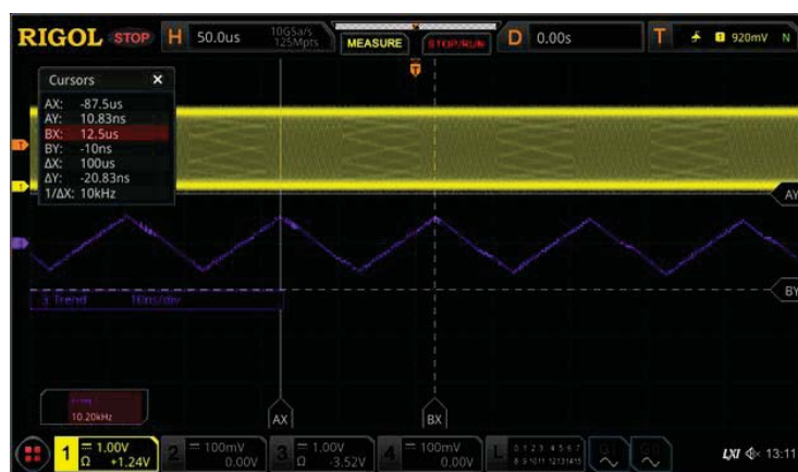
Figure 3: TIE trend graph cursor measurements
