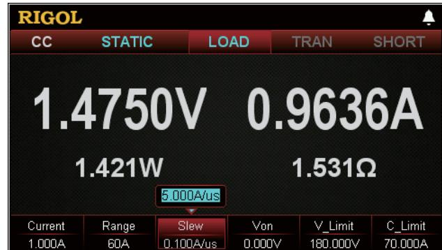
Current rising speed is defined as the speed of transition from one setting to another. You can set the actual transition time from one setting to another by changing the current rising speed. Adjustable current rising speed: 0.001 A/μs to 5 A/μs.
