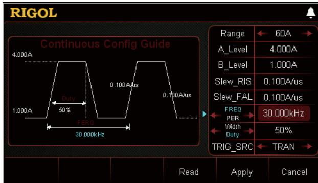
Transient test function enables the load to periodically switch between two set levels (Level A and Level B). It can be used to test the transient characteristics of the DUT. The highest frequency can be set to 30 kHz. Besides, in the guide interface, you can configure parameters in the parameter configuration list and view the configuration diagram at the left of the configuration list in the real-time manner.
