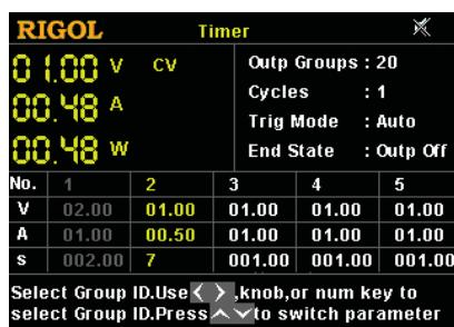
When the timing output is enabled, the system will configure the voltage, current, and the duration time based on the preset timer parameters, so as to provide varied voltage and/or current output for the load.
