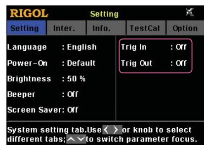
When multiple power supplies are in serial or parallel connection, enabling the external trigger function can realize the synchronous output for multiple power supplies.
