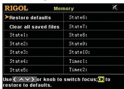
It supports storing and recalling state files and timer files, and allows you to restore the instrument settings to defaults.
