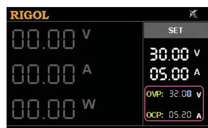
You can set thresholds for OVP and OCP values. If overvoltage or overcurrent occurs, the power supply shuts down the output automatically, and then a prompt message is displayed.
