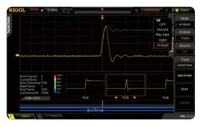
Serial bus trigger&decoding functions (RS232, I2C, SPI, and CAN)
