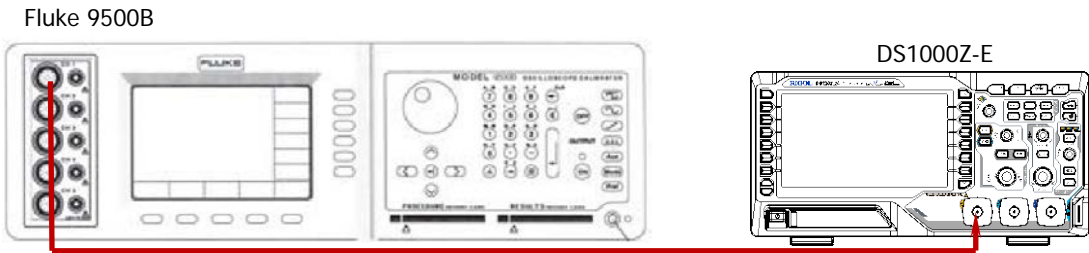
Figure 2-1 Impedance Test Connection Diagram
