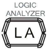
Press this key to open the logic analyzer control menu. You can turn on or off any channel or channel group, modify the display size of the digital channel, modify the logic threshold of the digital channel as well as group the 16 digital channels and display them as a bus. You can also set a label for each digital channel.
