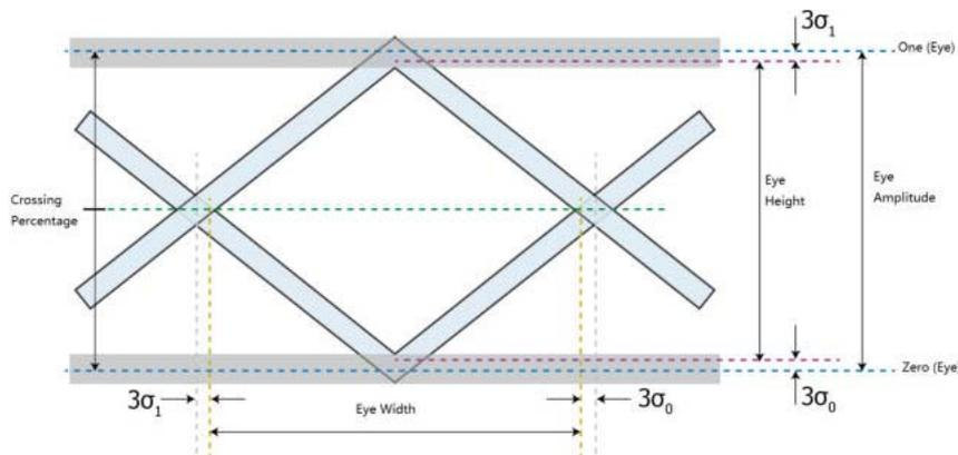
**Figure 12.3 Diagram of Eye Measurement Parameters**
