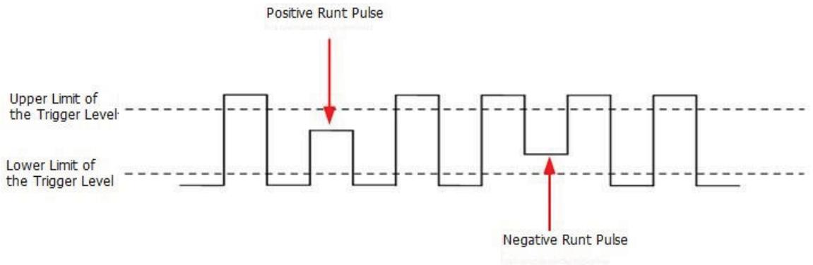
Figure 8.15 Runt Trigger
