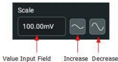
In the **Vertical** system menu, select **ON** or **OFF** to enable or disable the fine adjustment. By default, it is OFF. You can also press down the vertical scale knob on the small screen to enable or disable the fine adjustment.
