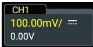
Click/tap the channel status label at the bottom of the screen or press the button
