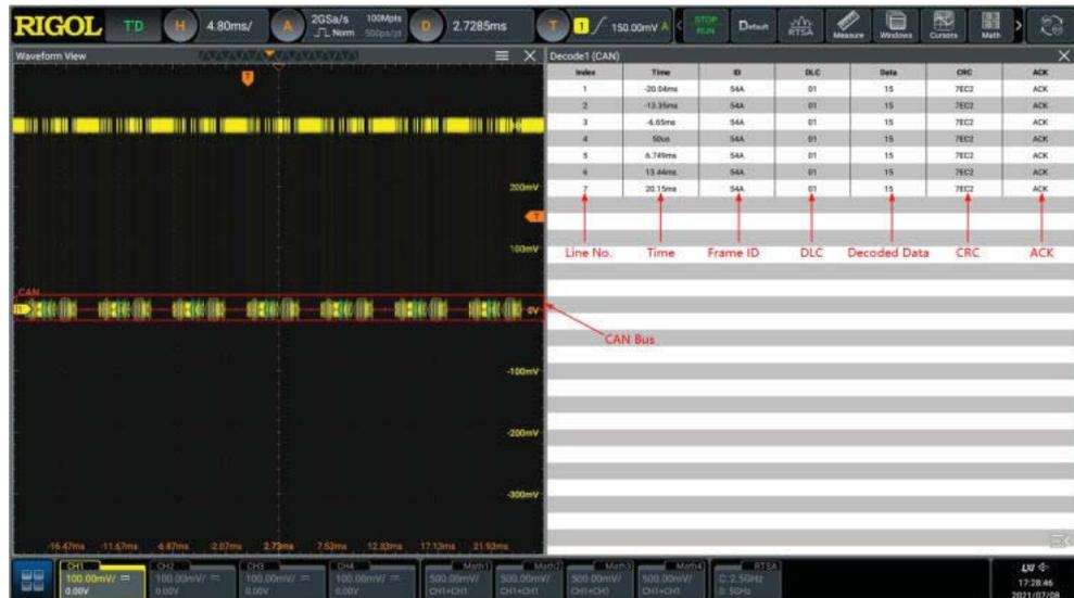
Figure 17.18 CAN Decoding Event Table
