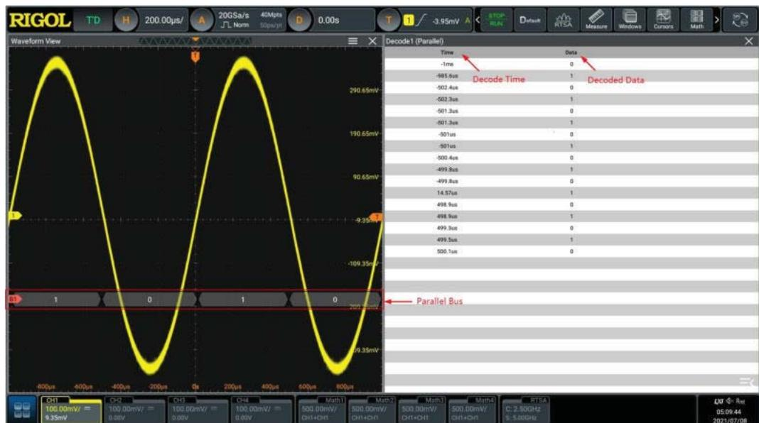
Figure 17.3 Parallel Decoding Event Table
