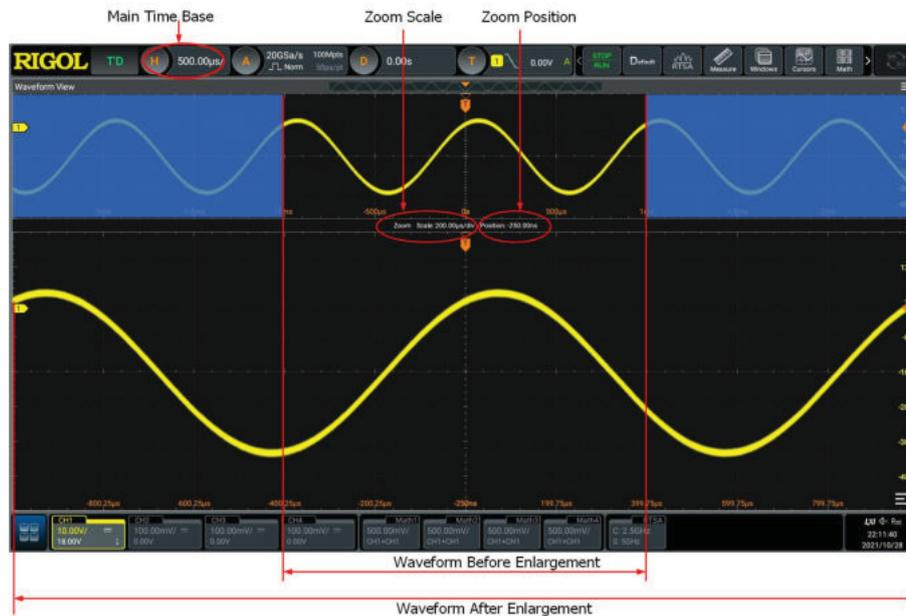
**Figure 6.2 Delayed Sweep Mode**
