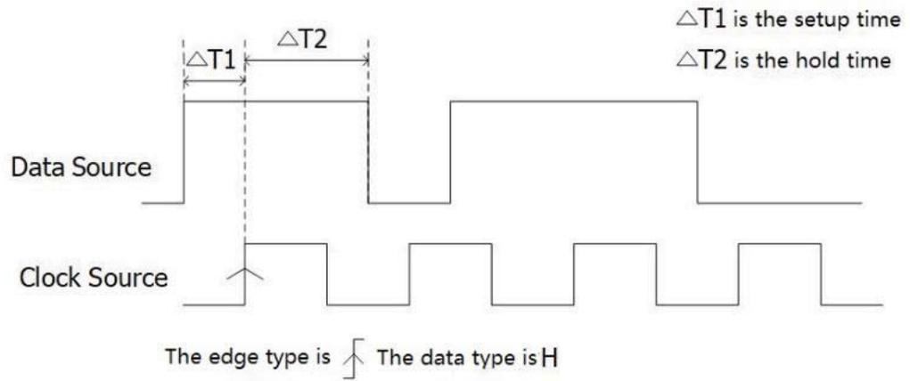
**Figure 8.20 Setup/Hold Trigger**
