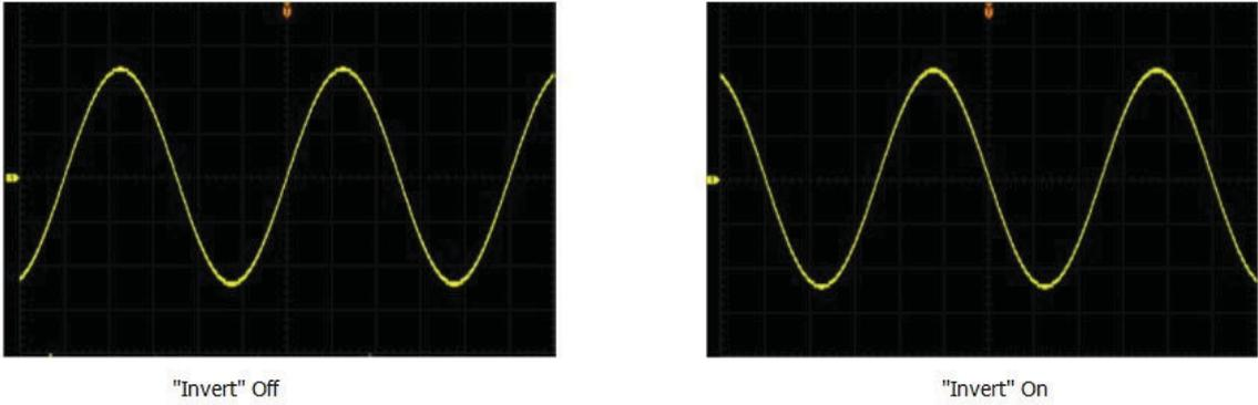
Figure 5.3 Waveform Invert
