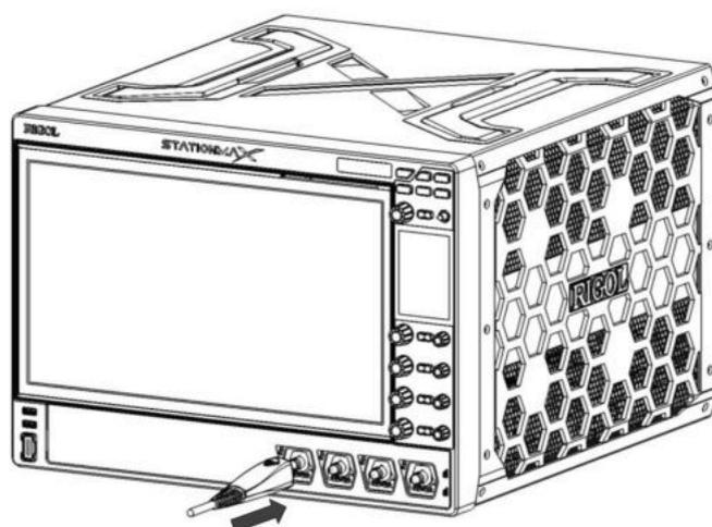
**Figure 4.6 To Connect the Active Probe**
