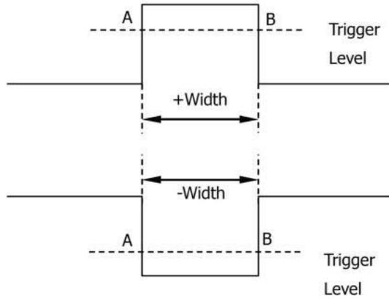
**Figure 8.4 Positive Pulse Width/Negative Pulse Width**
