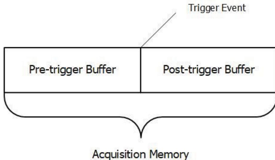
**Figure 8.1 Schematic Diagram of the Acquisition Memory**
