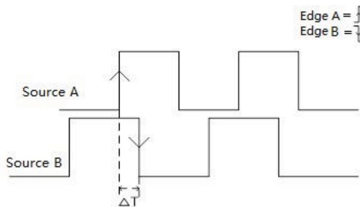
Figure 8.18 Delay Trigger
