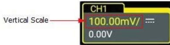
The adjustable range of the vertical scale is related to the currently set probe ratio and input impedance. By default, the probe ratio is 1X and the input impedance is 1 MΩ. In this case, the adjustable range of the vertical scale is from 1 mV/div to 10 V/div.
