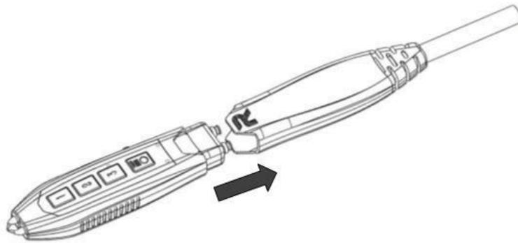
**Figure 4.5 To Connect the Probe Head to the PA of the Active Probe**
