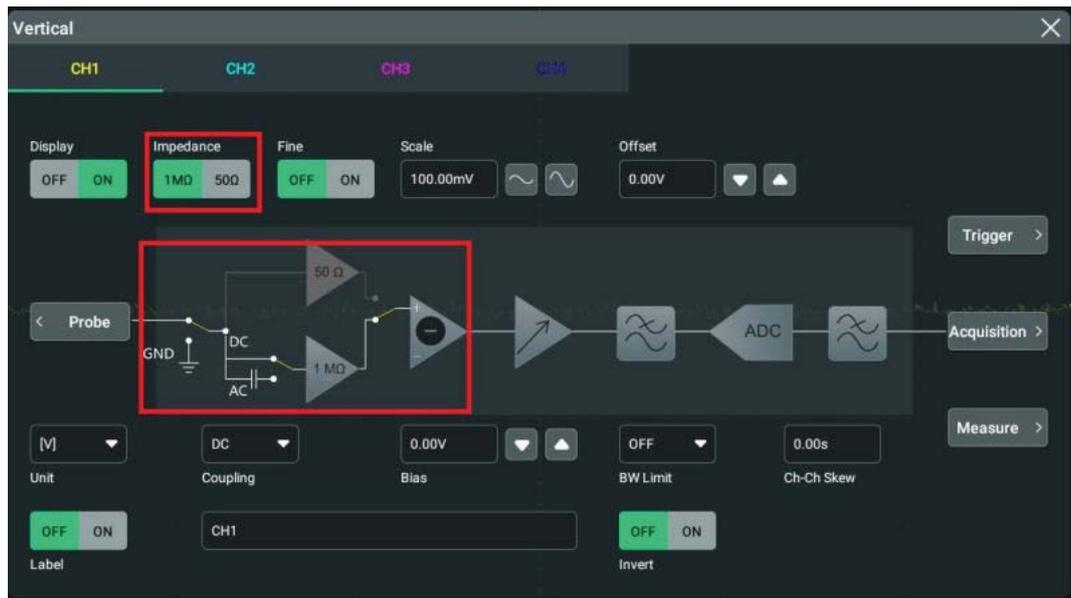
Figure 5.2 Input Impedance Modification
