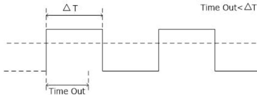
Figure 8.13 Timeout Trigger
