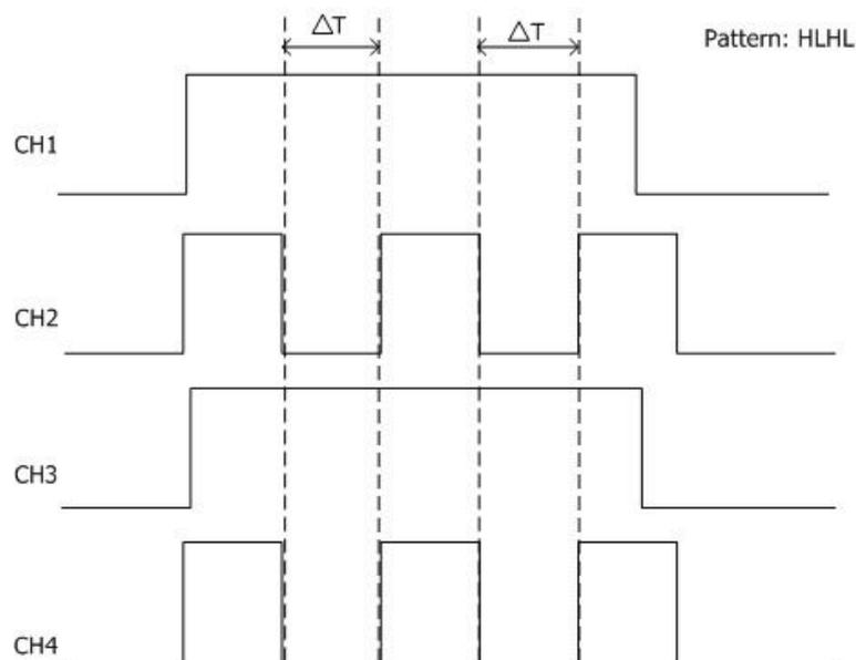
Figure 8.11 Duration Trigger
