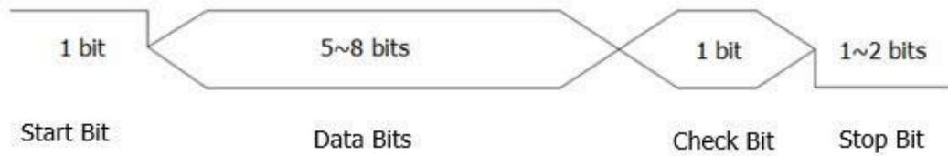
Figure 8.24 Schematic Diagram of RS232 Protocol
