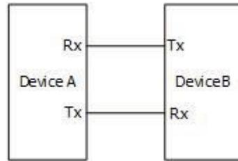
**Figure 17.4 Schematic Diagram of RS232 Serial Bus**
