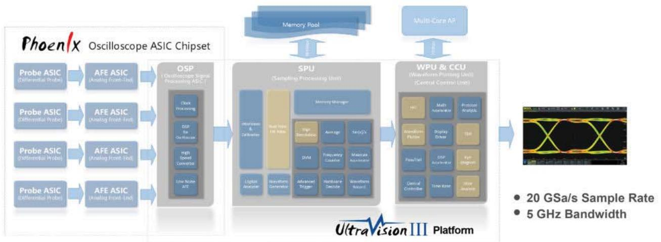
DS70000 series digital oscilloscope is equipped with "Phoenix" chip set, which delivers a max. of **20 GSa/s sample rate** and **5 GHz bandwidth** to better achieve signal fidelity, cover more application scenarios, and cater to the diversified application demands of the complex test system in the industry and R&D fields.
