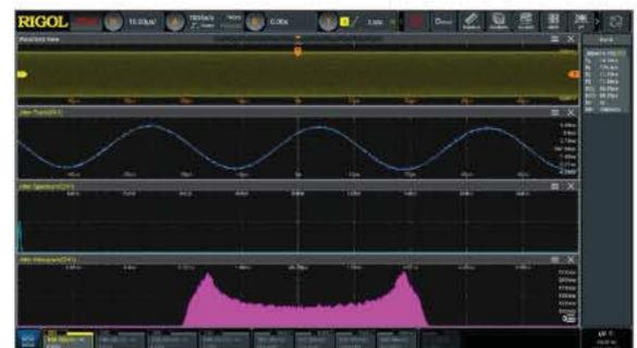
Perform TIE measurements on the clock signal with the jitter and analyze the results through the trend graph and histogram.
