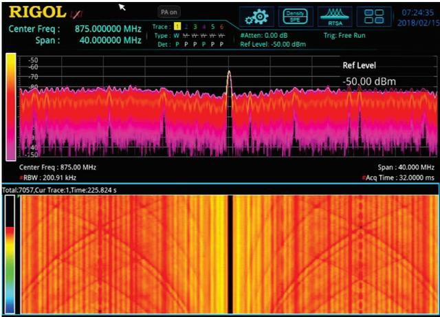
**Figure 9: Debugging emissions with the density display (top) and the spectrogram waterfall chart (bottom)**
