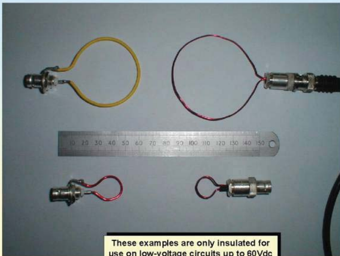
Figure 4 Examples of home-made unshielded loop probes
