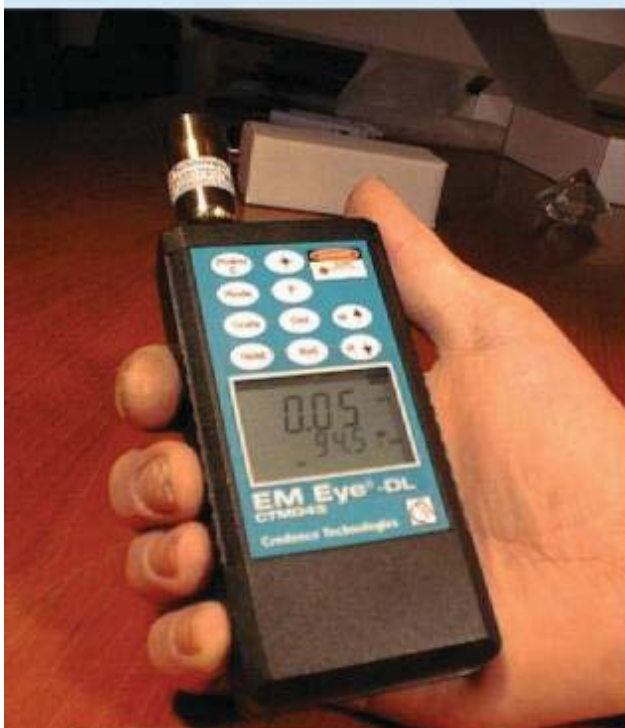
Battery-powered probe with directional antenna and LCD display of field strength in V/m
