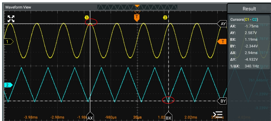
Figure 10.10 Track Measurement (before Horizontal Expansion)
