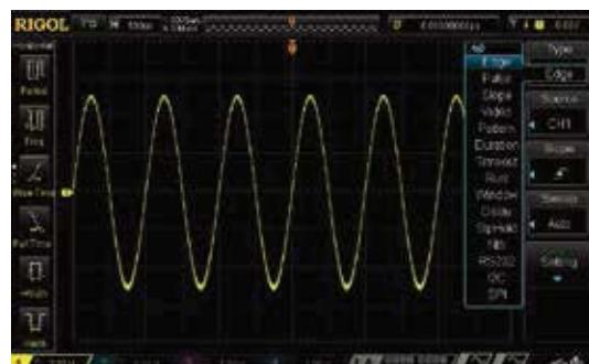
Optional serial bus trigger and decoding functions
