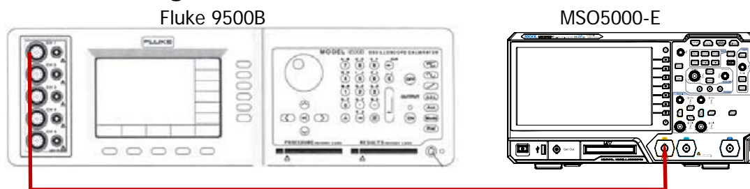
Figure 2-2 DC Gain Accuracy Test Connection Diagram
