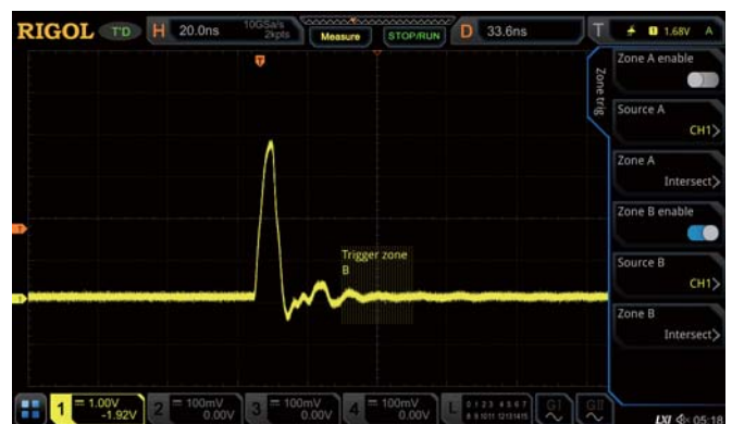
Quickly isolate the exceptional signal with Edge trigger and Zone trigger.
