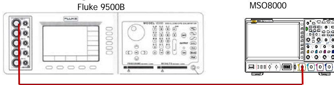
Figure 2-1 Impedance Test Connection Diagram
