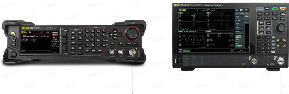
Figure 1: Signal Source + RSA6000 Spectrometer (Built-in ZigBee) combination
