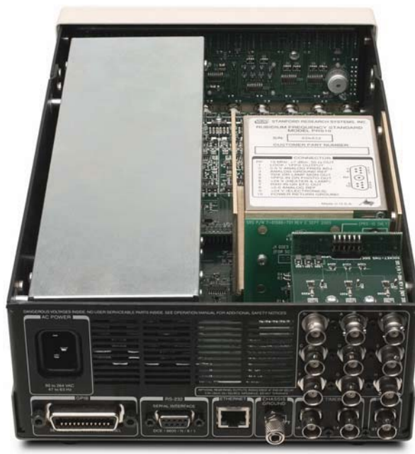
DG645 (cover removed) with optional Rb timebase. Rear panel shows the optional eight-channel outputs.
