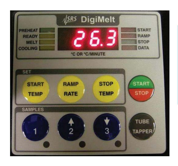
The keypad makes setting up a melt program very easy. The students push the yellow 'START TEMP' and then use the blue buttons with arrow keys to set the starting temperature. The students do the same for the 'RAMP RATE' and 'STOP TEMP' keys. Once the parameters are entered, they push the 'START/STOP' button and the microprocessor takes care of heating the block.
