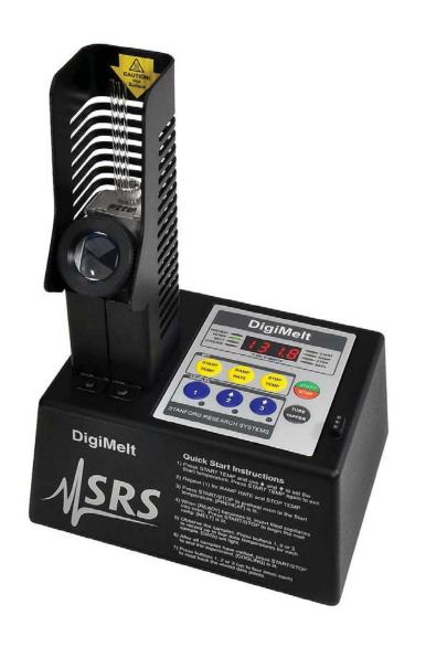
Student grade melting point apparatus
