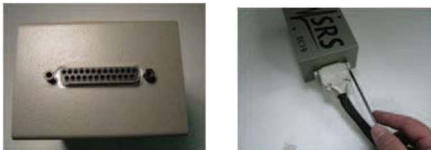
Figure 4: EC19 rear panel connector. Securing the umbilical cable.
