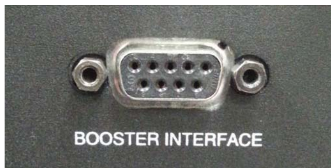
Figure 28: Rear panel connector for booster interface.
