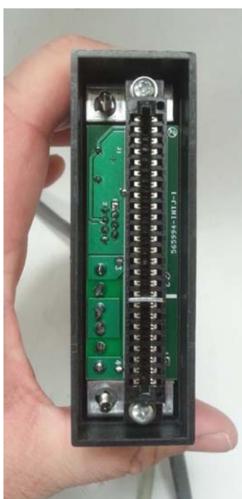
Figure 29: Interface card and edge connector for the external booster.
