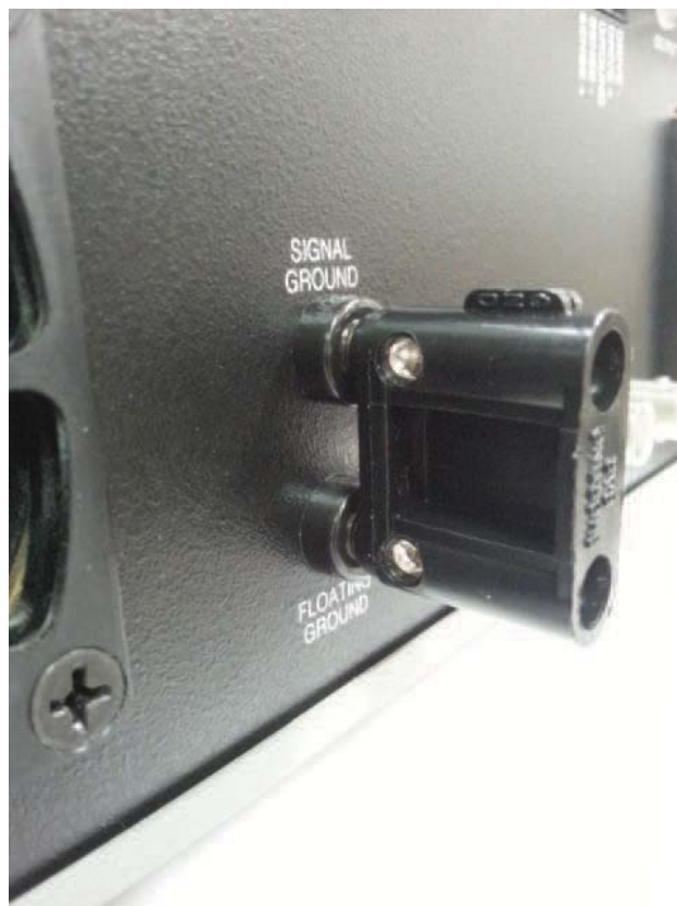
Figure 13: EC301 grounding bar (installed).
