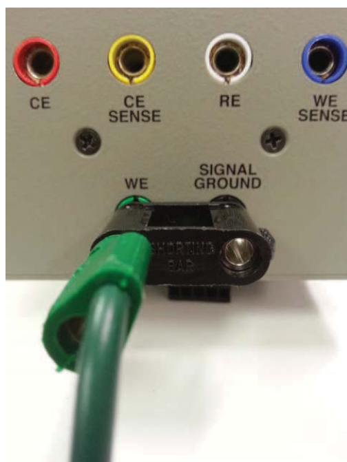
Figure 15: Grounding WE at the EC19.
